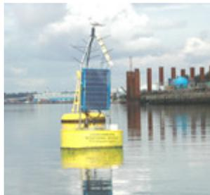
Five buoy-mounted automatic water quality monitors (AWQMs) have been installed by YSI Hydrodata engineers at the new Tyne Tunnel project to ensure that construction operations do not significantly affect river water quality.
